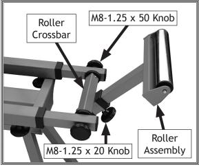
Figure 4. Support roller assembly.
